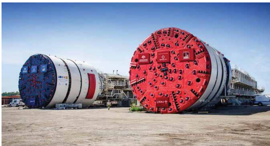
The tunnel boring machine PHOTO COURTESY BRISBANE CITY COUNCIL
