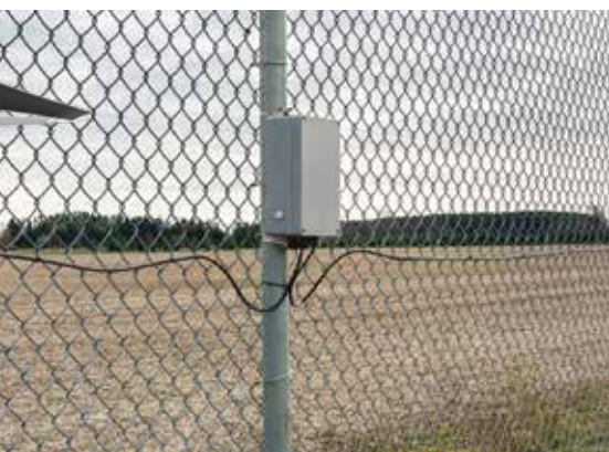
Senstar fence-mounted sensors detect and locate intruders at the fence line.
