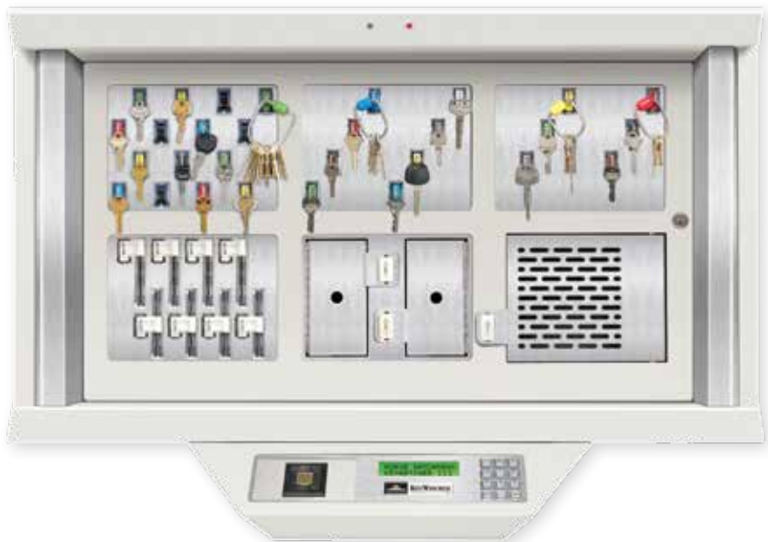
The MorseWatchmans KeyWatcher, a touchscreen electronic lockbox, shows who has a particular key and when it is due back. PHOTO COURTESY IST/MORSE WATCHMANS INCORPORATED-USA
