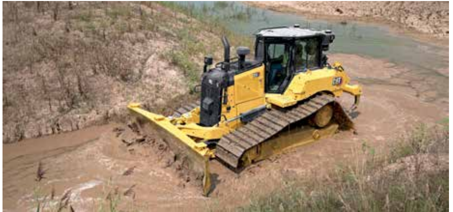
HawthorneCat's electric D6XE makes 100 percent of its torque at RPMs. PHOTO COURTESY HAWTHORNECAT
