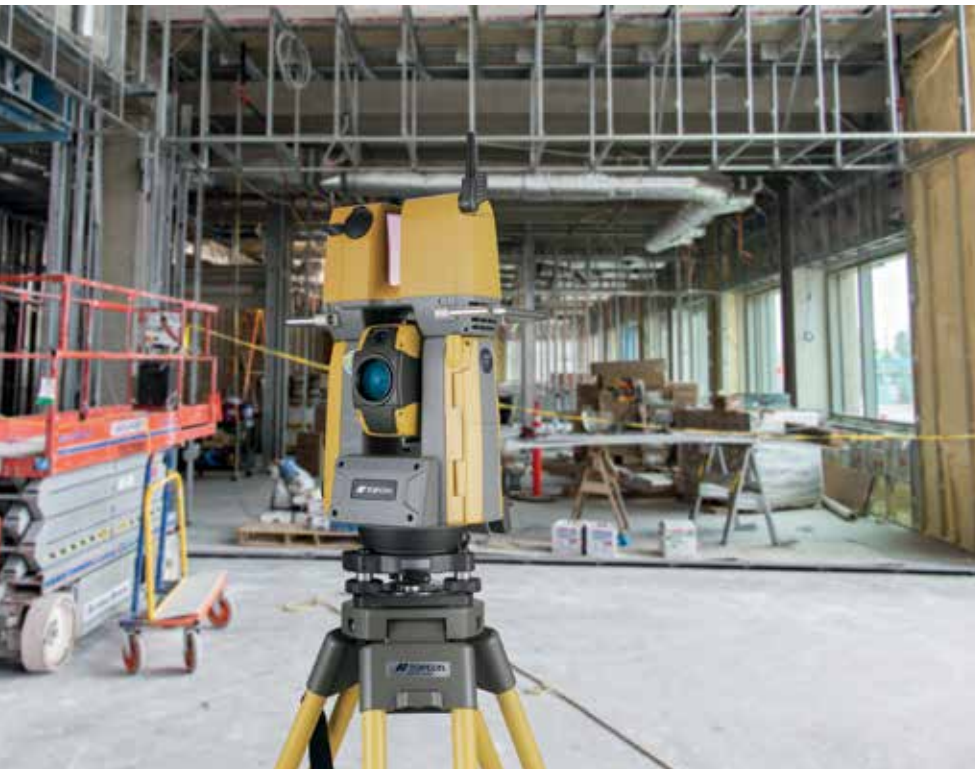
Topcon’s GTL-1000 scanner linked to a robotic total station PHOTO COURTESY TOPCON POSITIONING GROUP
