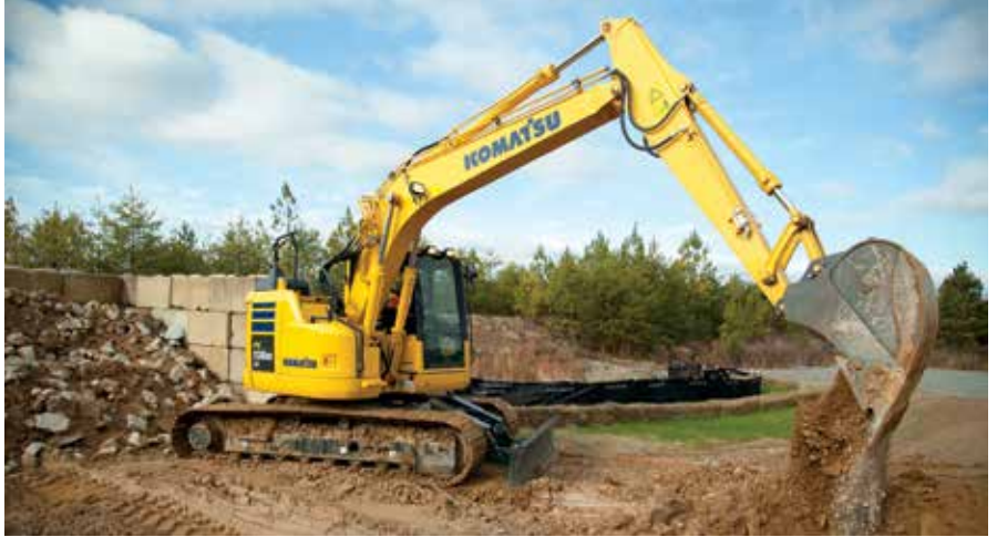
Komatsu’s PC138USLC hydraulic mini-excavator, a Bacon Universal best-seller, features a tight tail swing design. PHOTO COURTESY KOMATSU/BACON UNIVERSAL CO. INC.
