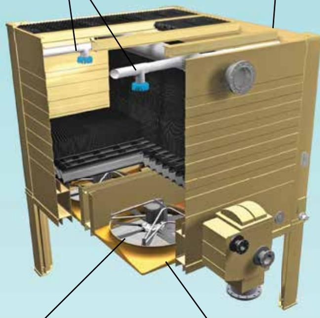
Direct-drive fans are located out of the corrosive airstream for double the service life.
