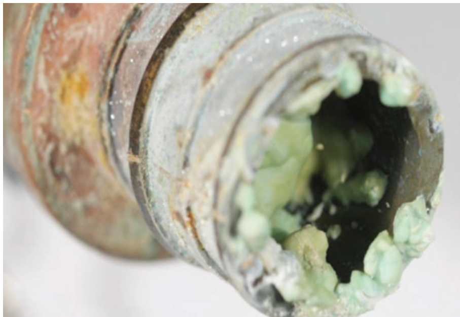
A PEX, yellow brass fitting, attaching the PEX tubing to a copper water line. The fitting is badly dezincified, with a substantial meringue deposit inside the fitting, as well as on the barbs which lie between the fitting and PEX tub.
