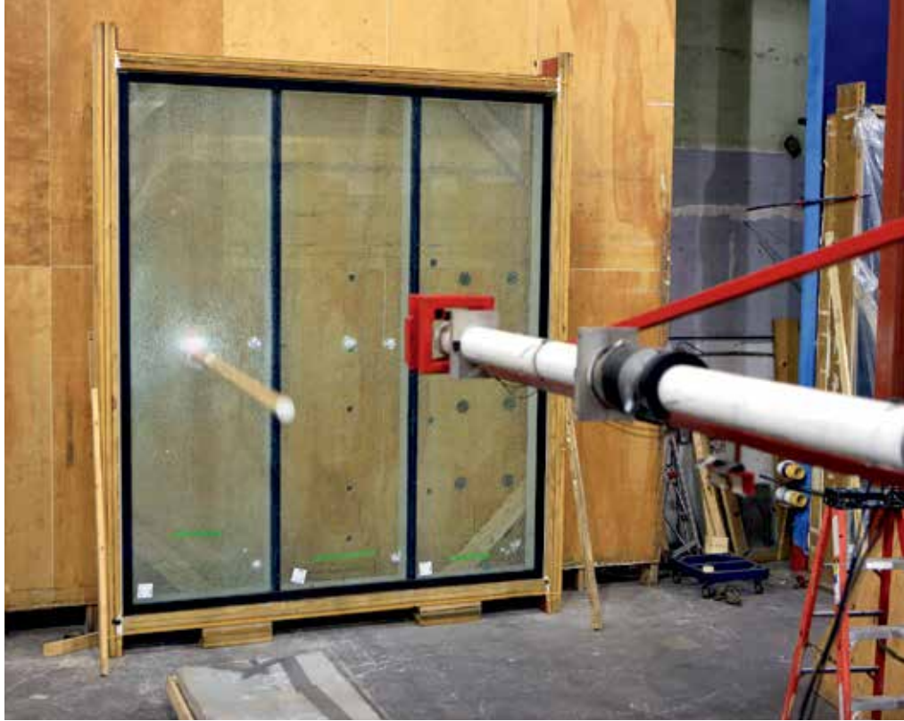
The large missile impact test for hurricane-resistant glass shoots a two-by-four traveling at 50 feet per second into a window.
