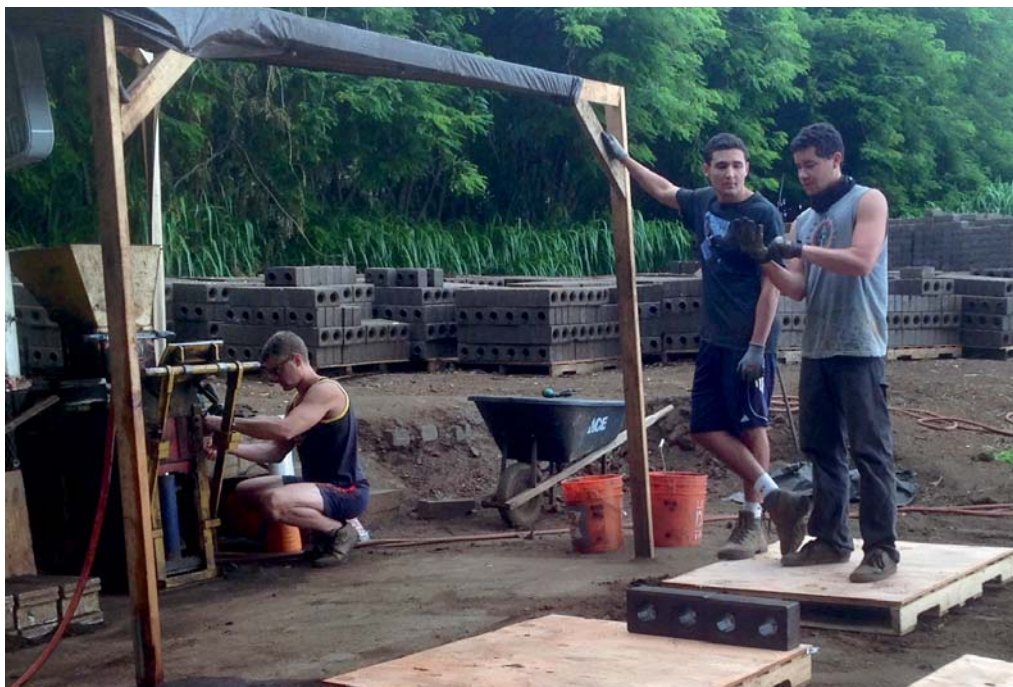
The crew manufactures mud bricks for the Martino home.
