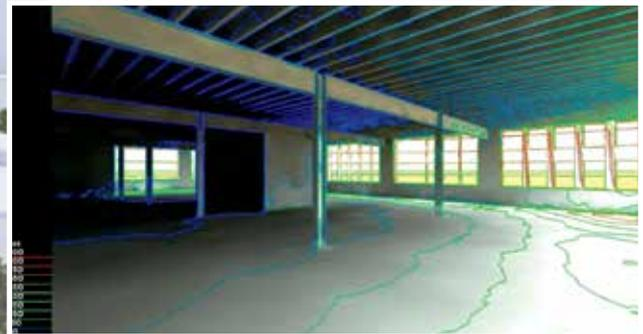
(above) Revit software features energy analysis providing information about daylight and shade; (left) A rendering created with Revit software RENDERINGS COURTESY AUTODESK
