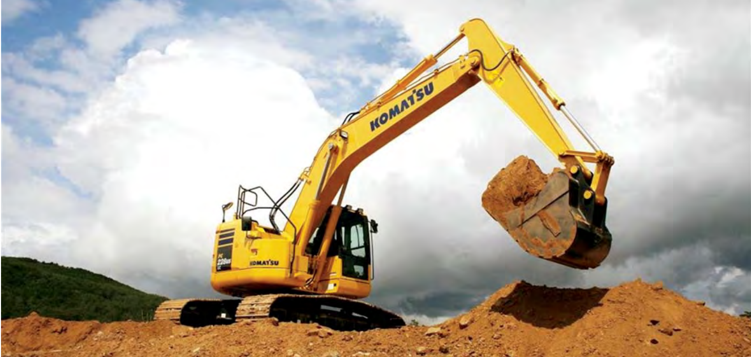
With its Zero Tail Swing design, Komatsu's PC228 is built to work in the tightest of spaces.
