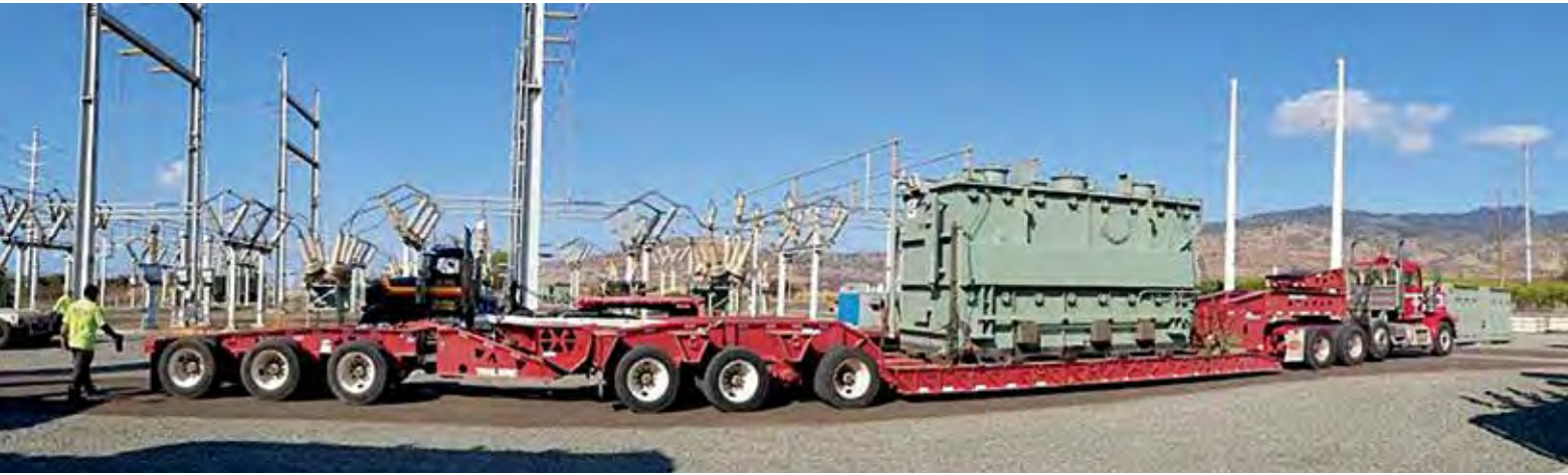
An 80-ton transformer was hauled by Yamashiro Trucking from Kapolei to Kaneohe. Hawaiian Crane and Rigging handled the loading and off-loading. PHOTOS COURTESY HAWAIIAN ELECTRIC CO.
