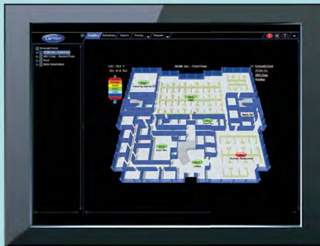
i-Vu® web-based control interface
