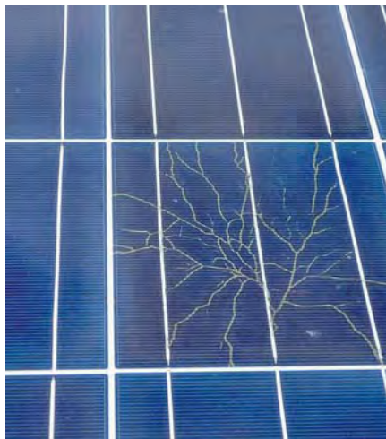
Damages might involve cracks in the panels.
