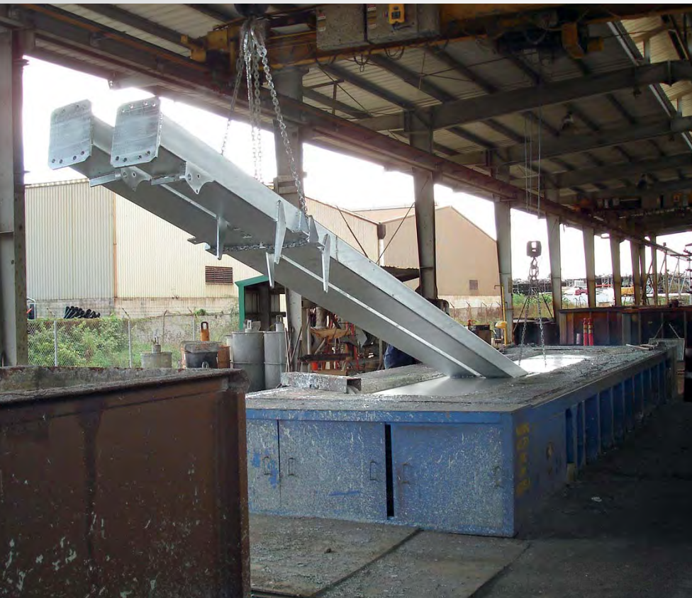
Steel columns are treated in a hot-dip galvanizing kettle at Kloeckner Metals.
