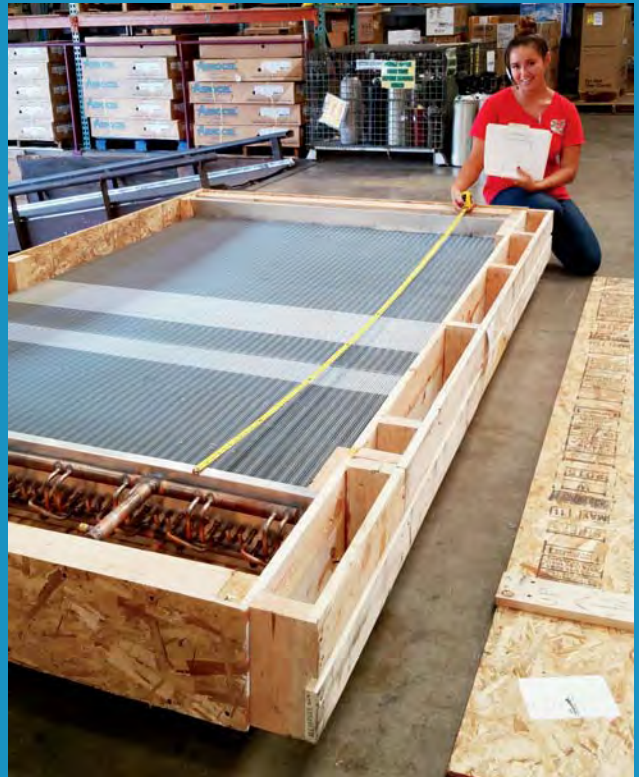
Cosco Hawaii designed a custom coil to replace the Kaiser High School band room condenser coil.
